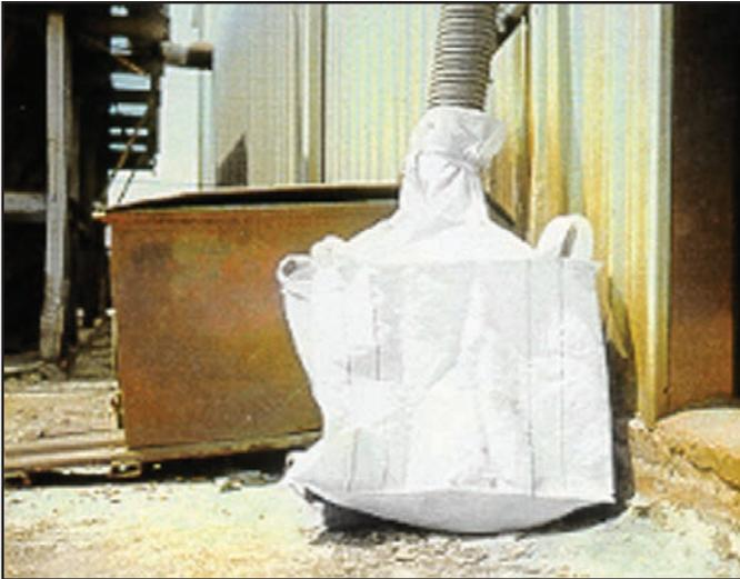
**A Simple, efficient means of collecting and removing unwanted residues produced during the blast process.**
