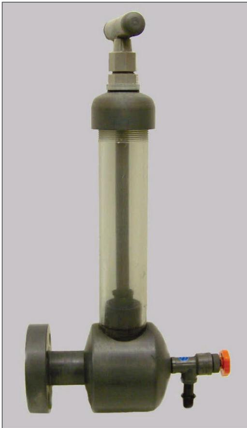
**Sample Pump:** Allows for a spill-free sample to be taken at the product line without the need to open the top of container system. The hand operated plunger allows for a spill free transfer from tank to sample bottle. Constructed of PVC, this user-friendly device can also be mounted unto any of our parallel instrument tees for sample draw applications.
