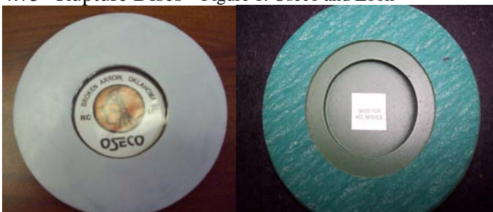
4.75” Rupture Discs - Figure 1. Oseco and Zook
