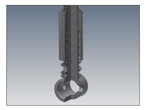
2) Assemble the eyebolts. Lubricate the nut with anti-seize and thread the nut onto the eyebolt in the orientation shown. Place the washer over the end of the eyebolt, then secure it by installing the e-clip into the slot on the end of the eyebolt. Repeat this three times.
