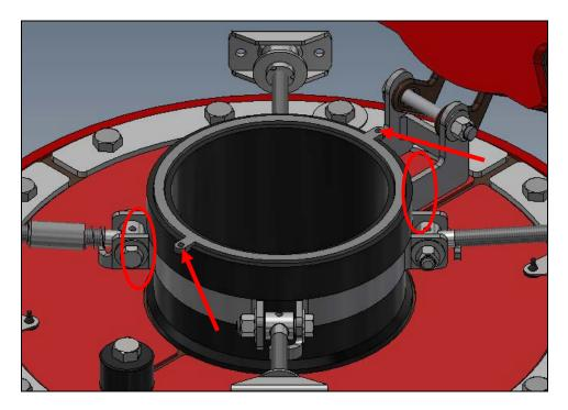
11) Close the fill cover and hand tighten the four eyebolts. Tool tighten the nuts an additional <sup>1</sup>/<sub>4</sub> to <sup>1</sup>/<sub>2</sub> turn. Customers may substitute their own torquing procedure as they see fit.
