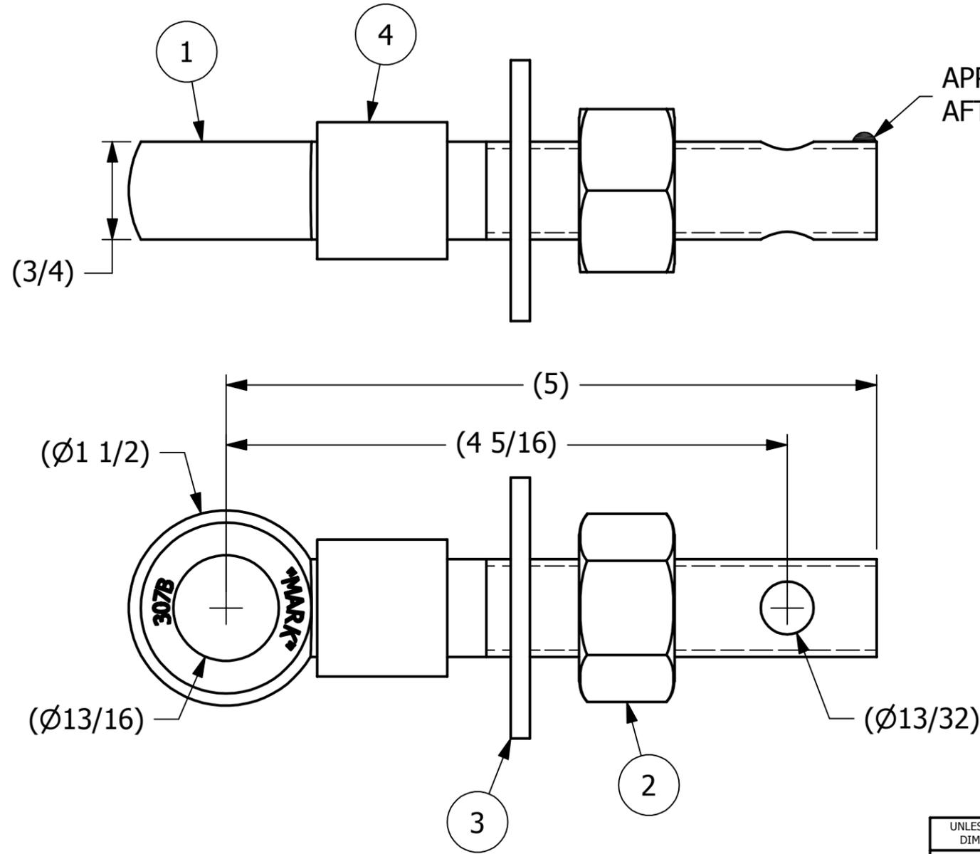
APPLY A BEAD OF WELD TO THE TWO END THREADS AFTER INSTALLING COLLAR, WASHER AND NUT.
