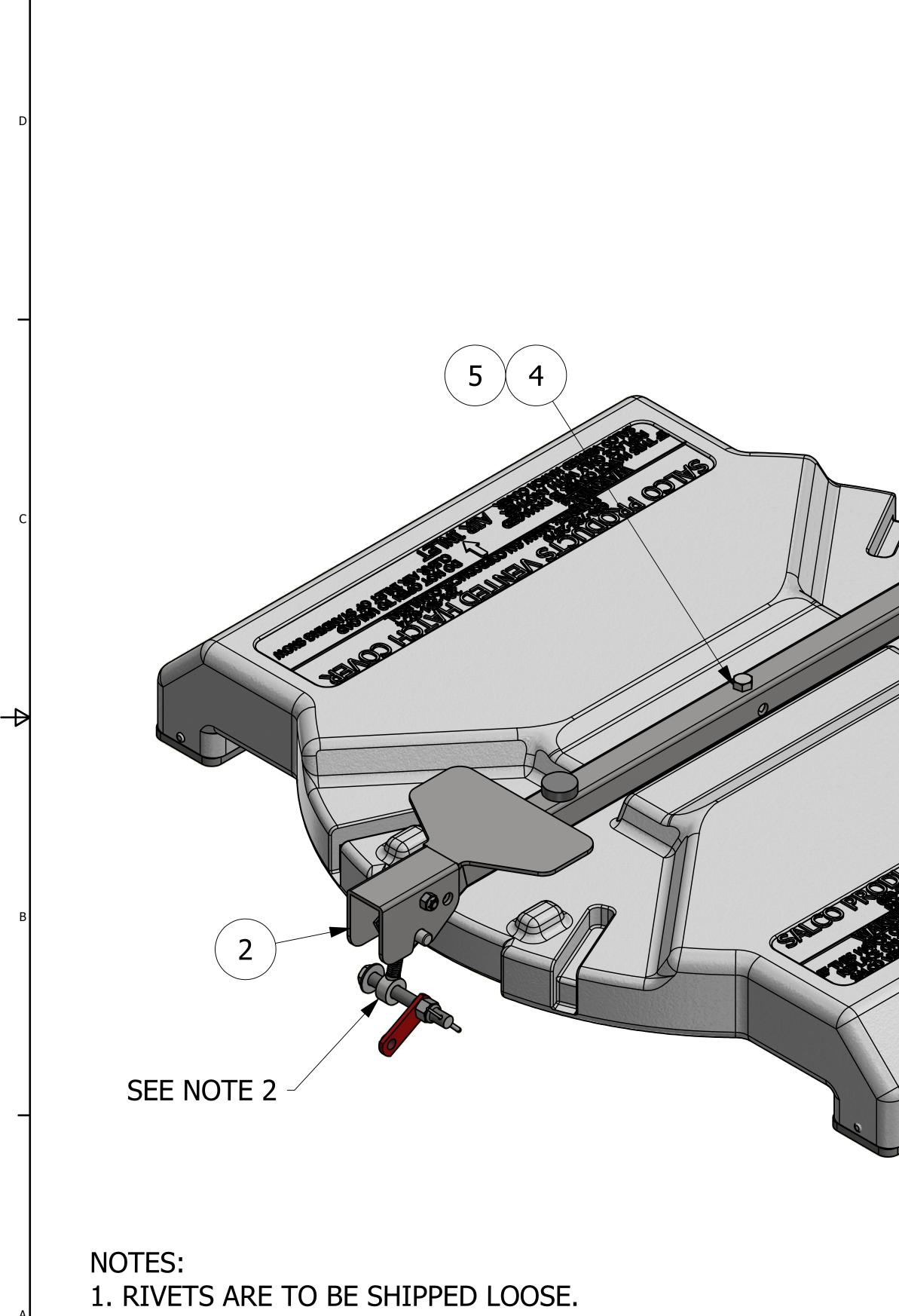
2. LOCTITE METAL-FREE TYPE ANTI SEIZE HAS BEEN APPLIED TO FOOT LATCH THREADS.
