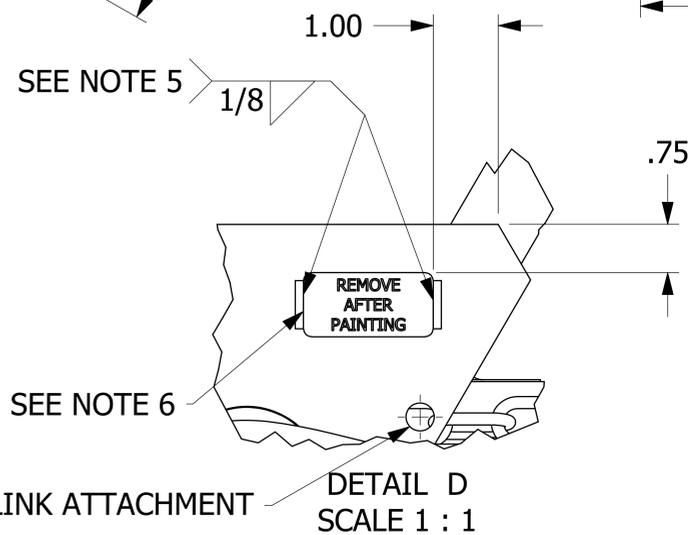
Ø7/16" HOLE FOR CHAIN LINK ATTACHMENT
